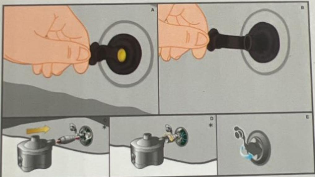
**GB Airbed:** A/ Open the valve. B/ Pull the external stopper to extend the valve out. C/ Attach adapter nozzle of the pump to the airbed valve by twisting it gently. Turn on the pump\* to inflate. D/ When fully inflated, seal valve by pushing in with pump nozzle. Gently twist adapter sleeve to right removing the pump from the valve while maintaining the seal. E/ Close the external stopper. Valve should appear depressed into itself.
